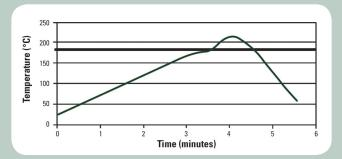
Peak reflow temperature should be <340°C in a nitrogen atmosphere (<100ppm  $0_2$ ), with a linear ramp up to 30°C above liquidus temperature. These profiles are recommended to the user as starting points, and should be optimized by the user to meet their individual process needs.
