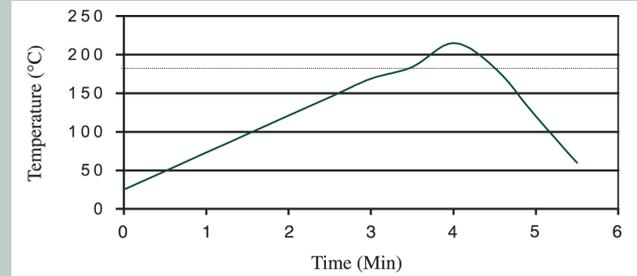
The profile shown here is designed for **Indium6.2** with Sn63/Pb37 and Sn62/Pb36/Ag2 under both air and nitrogen reflow atmospheres. It serves as a general guideline in establishing a reflow profile for these alloys.
