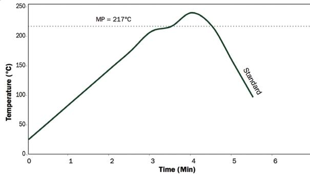
Indium6.6HF-HD should be reflowed using a linear profile in an air or nitrogen atmosphere. The stated profile recommendations can be used as a general guideline in establishing a reflow profile for Indium6.6HF-HD with SnAgCu, SnAg, and SnSb alloy systems.
