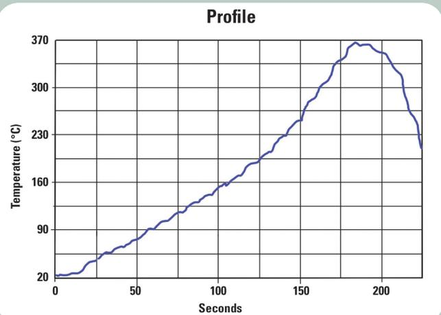
The profile above is designed for use with Durafuse® HT in a nitrogen atmosphere or forming gas (<100ppm O<sub>2</sub>). Recommended peak temperature is 350–385°C. It can serve as a general guideline for establishing a profile for your process and should be regarded as a typical example. Adjustments to this profile may be necessary based on assembly size, thermal density, and other factors.
