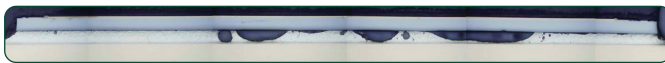
0.2µm Ni – cross section of the voids revealed Ni leaching and interfacial de-wetting.
