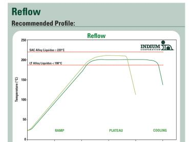
This profile is designed for use with **Durafuse® LT with SiPaste® C201HF**. This can be used as a general guideline in establishing a reflow profile for **Durafuse® LT** Solder Paste. Deviations from these recommendations are acceptable, and may be necessary, based on specific process requirements.
