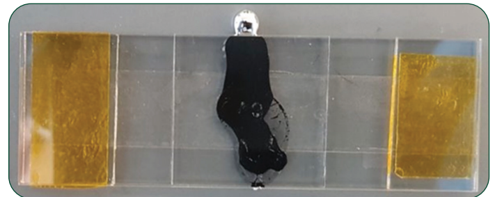
Standard gallium-based liquid metals do not spread isotopically when under pressure.
