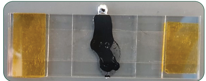
Standard gallium-based liquid metals do not spread isotopically when under pressure.
