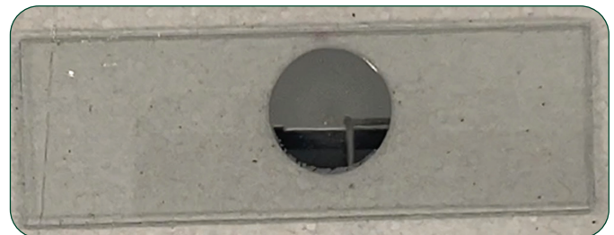
LMP: Due to its higher viscosity, liquid metal paste will spread isotopically.
