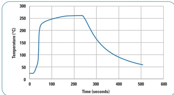
Figure 5. Sinter profile: 3 minutes, 250°C @ 20MPa.
