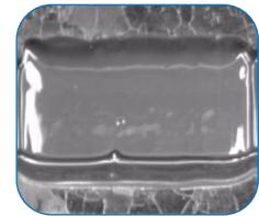
Figure 3. Dog-eared edges due to excessive separation speed.
