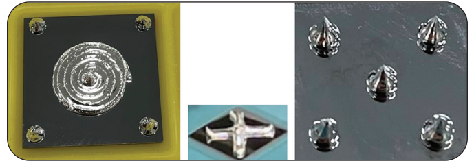
Figure 4. Examples of liquid metal paste in a variety of dispense patterns.
