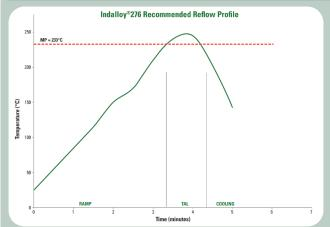
This can be used as a general guideline in establishing a reflow profile when using **Indium8.9HF with Indalloy®276 Solder Paste**. Deviations from these recommendations are acceptable, and may be necessary, based on specific process requirements, including board size, thickness, and density. Start with a linear profile. If needed, a flat soak portion or a linear shoulder may be added to reduce the thermal gradient.
