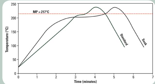
The stated profile recommendations apply to most Pb-free alloys in the SnAgCu (SAC) alloy system, including SAC305 (96.5Sn/3.0Ag/0.5Cu). This can be used as a general guideline in establishing a reflow profile when using Indium5.1 Solder Paste. Deviations from these recommendations are acceptable, and may be necessary, based on specific process requirements, including board size, thickness, and density.
