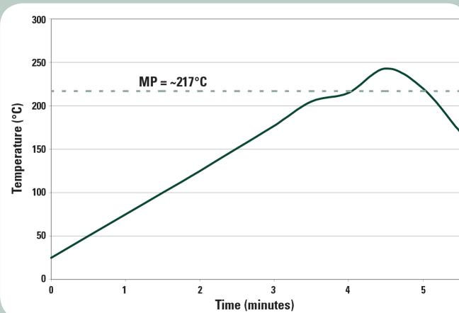
The above reflow profile was designed to serve as a starting point for process optimization using **Indium3.1 Solder Paste**. When seeking to minimize thermal gradient or reduce voiding in BGA assemblies, a profile utilizing a soak of up to 2 minutes at 205–210°C may help.
