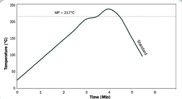
SiPaste® 3.2HF should be reflowed using a linear profile in an air or nitrogen atmosphere. The stated profile recommendations can be used as a general guideline in establishing a reflow profile for SiPaste® 3.2HF with SnAgCu, SnAg, and SnSb alloy systems.
