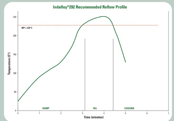
This can be used as a general guideline in establishing a reflow profile when using **Indium8.9HF with Indalloy®292 Solder Paste**. Deviations from these recommendations are acceptable, and may be necessary, based on specific process requirements, including board size, thickness, and density. Start with a linear profile. If needed, a flat soak portion or a linear shoulder may be added to reduce the thermal gradient.
