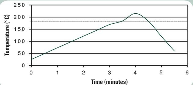
This profile is designed for use with Indalloy®205 (60In/40Pb) MP 181°C and Indalloy®227 (77.2Sn/20In/2.8Ag) MP 187°C. It will serve as a general guideline in establishing a reflow profile for your process. Adjustments to this profile may be necessary based on specific process requirements and the use of alloys with different melting temperatures.
