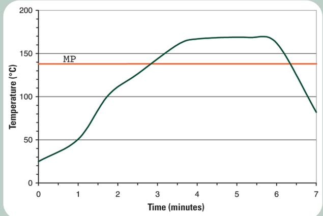
This profile is designed for use with Indalloy®282 and can serve as a general guideline in establishing a reflow profile for use with other alloys. Adjustments to this profile may be necessary based on specific process requirements.
