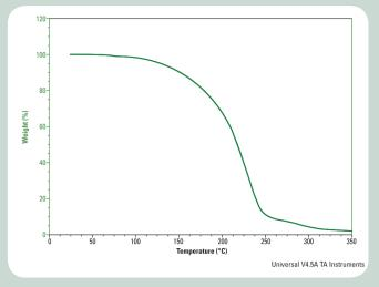
TGA was performed at a ramp rate of 10°C per minute.
