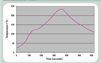
Flip-Chip Flux NC-699 is intended to be used in a nitrogen reflow environment of 100ppm oxygen or less. Some applications can utilize this material in an air environment, although best results will be obtained in an inert atmosphere. Flip-Chip Flux NC-699 can be used on many surface finishes including immersion Ag, Cu, and AuNi. These surfaces can be soldered with Pb-free alloys, but require nitrogen if reflow temperatures exceed 240°C.
