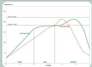
This profile is designed for use with Sn63/Pb37 and Sn62/Pb36/Ag2 and can serve as a general guideline in establishing a reflow profile for use with other alloys. Adjustments to this profile may be necessary based on specific process requirements. Start with the linear profile, then move to the optional soak profile, if needed.
