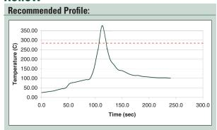
The typical profile above is designed for use with high-Pb (lead content 80% or greater) alloys in a forming gas or nitrogen atmosphere. This profile can serve as a general guideline for establishing a profile for your process and should be regarded as a typical example. Adjustments to this profile may be necessary based on assembly size, thermal density, and other factors. Use of other alloys with lower or higher liquidus temperatures will also require changes.
