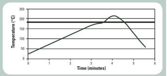
Peak reflow temperature should be <250°C in an air or nitrogen atmosphere, with a linear ramp up to approximately 30°C above the solidus temperature.
