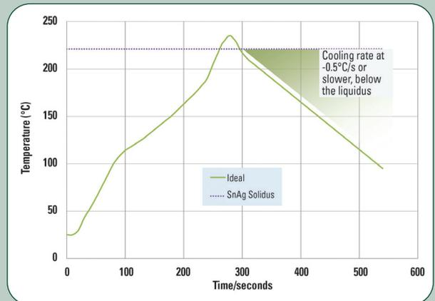
Profile optimized for thin die/thin substrate flip-chip.
