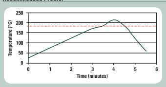
This profile is designed for use with Sn63/Pb37 and Sn62/Pb36/Ag2 and can serve as a general guideline in establishing a reflow profile for use with other alloys. Adjustments to this profile may be necessary based on specific process requirements.
