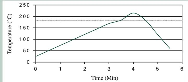
The profile shown here is designed for **Indium6.2** with Sn63/Pb37 and Sn62/Pb36/Ag2 under both air and nitrogen reflow atmospheres. It serves as a general guideline in establishing a reflow profile for these alloys.
