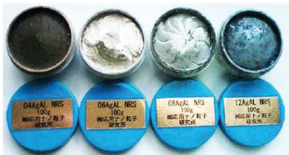
Figure 20. Examples of pastes based on alcoxide-stabilized nano-silver.
