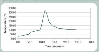
The typical profile above is designed for use with Sn10/Pb88/Ag2 or Sn5.0/Pb92.5/Ag2.5 alloy in a nitrogen atmosphere (500ppm oxygen or less). It can serve as a general guideline for establishing a profile for your process and should be regarded as a typical example. Adjustments to this profile may be necessary based on assembly size, thermal density, and other factors. Use of other alloys with lower or higher liquidus temperatures will also require changes.
