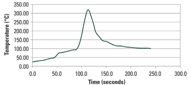
The typical profile above is designed for use with Sn10/Pb88/Ag2 or Sn5.0/Pb92.5/Ag2.5 alloy in a nitrogen atmosphere (500ppm oxygen or less). It can serve as a general guideline for establishing a profile for your process and should be regarded as a typical example. Adjustments to this profile may be necessary based on assembly size, thermal density, and other factors. Use of other alloys with lower or higher liquidus temperatures will also require changes.
