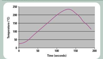
Flip-Chip Flux NC-26-A is intended to be used in a nitrogen reflow environment of 100ppm oxygen or less. Some applications can utilize this material in an air environment, although best results will be obtained in an inert atmosphere. Flip-Chip Flux NC-26-A can be used on many surface finishes including immersion Ag, Cu, and AuNi. These surfaces can be soldered with SnPb or Pb-free alloys, but require nitrogen if reflow temperatures exceed 240°C.
