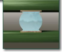
paste itself. The area ratio of the stencil apertures plays a large role in the transfer efficiency of the solder paste.
