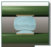
pump-out. Printing too fast or too slow will alter the amount of solder that is printed, as well as pulling the solder paste out of the apertures (scooping). Stencil design is probably the most important issue as a bad stencil
