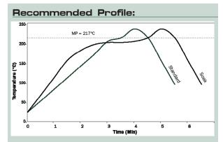
The stated profile recommendations apply to most Pb-free alloys in the SnAgCu (SAC) alloy system, including SAC 305 (96.5Sn/3.0Ag/0.5Cu). This can be used as a general guideline in establishing a reflow profile when using **Indium3.1AF** solder paste. Deviations from these recommendations are acceptable, and may be necessary, based on specific process requirements, including board size, thickness & density.
