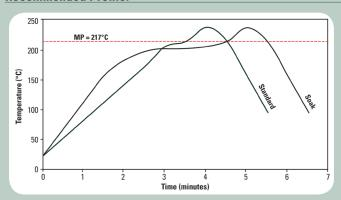
The stated profile recommendations apply to most Pb-free alloys in the SnAgCu (SAC) alloy system, including SAC305 (96.5Sn/3.0Ag/0.5Cu). This can be used as a general guideline in establishing a reflow profile when using **Indium3.1AF** Solder Paste. Deviations from these recommendations are acceptable, and may be necessary, based on specific process requirements, including board size, thickness, and density.
