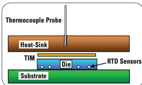
Figure 2. Schematic of TIM thermal test vehicle.
