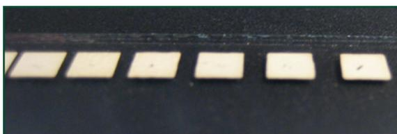
When the resistance (Ohm) is plotted with distance, a line is obtained. The intercept of the line to the y-axis is the theoretical resistance without a gap (without the sheet resistance factor of TCO).
