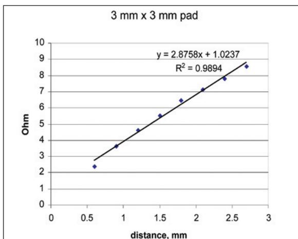
Contact resistance is calculated by multiplying the intercept (1.0237 Ohm) by the pad area (0.3cm x 0.3cm) divided by 2 (the number of pads).
