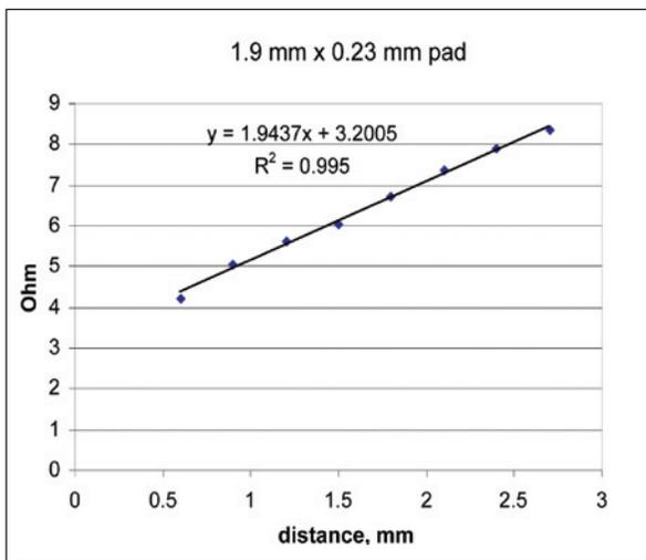
Contact resistance (contact resistivity) =  $3.2005 \text{ Ohm} \times 0.19\text{cm} \times 0.023\text{cm} / 2 = 0.007\Omega\text{cm}^2$  ( $7\text{m}\Omega\text{cm}^2$ ).
