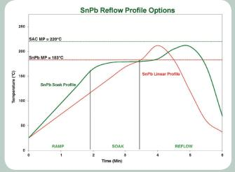
Peak reflow temperature should be <250°C in an air or nitrogen atmosphere, with a linear ramp up to approximately 30°C above the solidus temperature.
