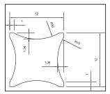
Aperture design for void reduction Screen material: SD 245/65 mesh at 22°, plus 200 um emulsion
