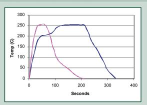
Users should define a suitable vacuum reflow profile that minimizes voids, reduces intermetallic formation, gives good residue cleanability, reduces die skew and die shift, and has good wetting onto metal surfaces.
