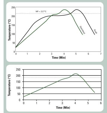
Peak reflow temperature should be  $<260^{\circ}$ C in an air or nitrogen atmosphere (<500ppm O<sub>2</sub>), with a linear ramp up to 30°C above liquidus temperature. These profiles are recommended to the user as starting points, and should be optimized by the user to meet their individual process needs.
