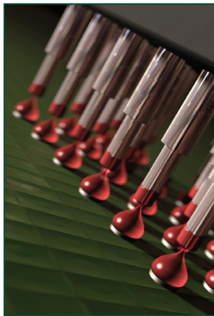
In addition to process and equipment variables, the working life of a flux can also affect the volume of flux that is transferred over time, and because flux is thixotropic, its viscosity can change with shear stresses.
