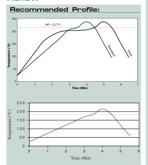
Peak reflow temperature should be <350°C in an air or nitrogen atmosphere (<500ppm  $^{\circ}$ ), with a linear ramp up to 30°C above liquidus temperature. These profiles are recommended to the user as starting points, and should be optimized by the user to meet their individual process needs.
