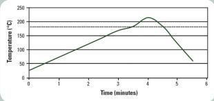
Peak reflow temperature should be <350°C in an air or nitrogen atmosphere (<500ppm  $0^2$ ), with a linear ramp up to 30°C above liquidus temperature. These profiles are recommended to the user as starting points, and should be optimized by the user to meet their individual process needs.
