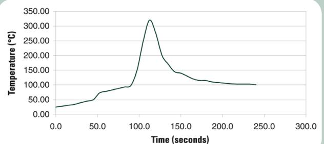
The typical profile above is designed for use with Sn10/Pb88/Ag2 or Sn5/Pb92.5/Ag2.5 alloy in a nitrogen atmosphere (500ppm oxygen or less). It can serve as a general guideline for establishing a profile for your process and should be regarded as a typical example. Adjustments to this profile may be necessary based on assembly size, thermal density, and other factors. Use of other alloys with lower or higher liquidus temperatures will also require changes.
