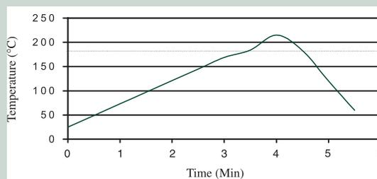
The profile shown here is designed for **Indium6.2** with Sn63/Pb37 and Sn62/Pb36/Ag2 under both air and nitrogen reflow atmosphere. It serves as a general guideline in establishing a reflow profile for these alloys.
