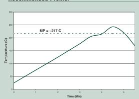
The above reflow profile was designed to serve as a starting point for process optimization using **Indium3.1**. When seeking to minimize thermal gradient or reduce voiding in BGA assemblies, a profile utilizing a soak of up to 2 minutes at 205-210°C may help.
