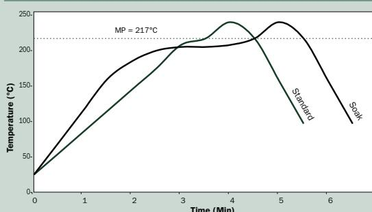
The stated profile recommendations apply to most Pb-Free alloys in the Sn/Ag/Cu (SAC) alloy system, including SAC 305 (96.5Sn/3.0Ag/0.5Cu). This can be used as a general guideline in establishing a reflow profile when using **Indium5.1AT** Solder Paste. Deviations from these recommendations are acceptable, and may be necessary, based on specific process requirements, including board size, thickness & density.
