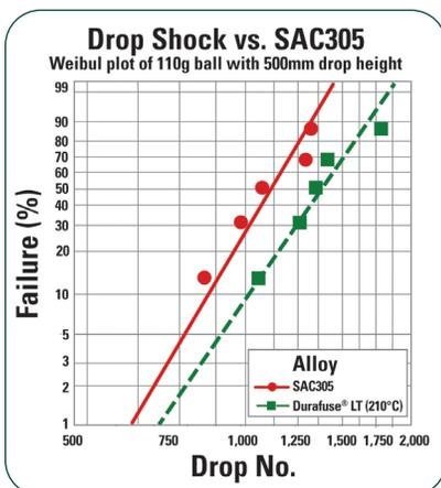
**Durafuse<sup>®</sup> LT** samples in the chart (left) experienced a peak reflow temperature of 210°C and demonstrated drop shock resilience similar to that of SAC305.
