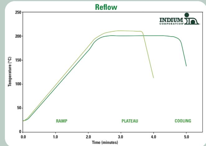
This profile is designed for use with **Durafuse® LT** in Indium5.7LT-1. This can be used as a general guideline in establishing a reflow profile for **Durafuse® LT** Solder Paste. Deviations from these recommendations are acceptable, and may be necessary, based on specific process requirements.
