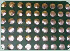
Hole Fill Test Board
