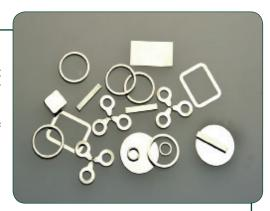
Indium Corporation's unique coating process can control the amount of flux to tight tolerances. Flux coatings are measured and applied by weight percentage. The standard weight percentage ranges from 1–3%  $\pm$  0.5%. The flux coating is applied after the dimensions of the preform have been verified.
