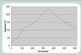
WS-446HF Flip-Chip Flux is intended to be used in a nitrogen reflow environment of 50ppm oxygen or less. Some applications can utilize this material in an air environment, although best results will be obtained in an inert atmosphere. WS-446HF Flip-Chip Flux can be used on many surface finishes.
