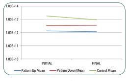
The electromigration test is performed to IPC-TM-650 method 2.6.14.1 with boards prepared using IPC-TM-650 method 2.6.3.3. The test conditions for this test are 496 hours at 65°C  $\pm$ 2°C and 88.5%  $\pm$ 3.5% RH. To pass this test, there should be no visible corrosion and no dendritic growth that decreases line
