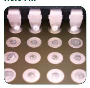
Indium Corporation uses several of its own tests, based on IPC workmanship standards, for determining hole fill. Depending on the design criteria for the flux, Indium Corporation uses holes of varying sizes and circuit board finishes. However, we always look for 100%
