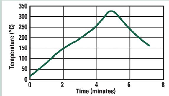
This profile is for use with Indalloy®151 (92.5Pb/5Sn/2.5Ag) and Indalloy®163 (95.5Pb/2Sn/2.5Ag) alloys and will serve as a general guideline in establishing a reflow profile for your process. Adjustments will be necessary for use with other alloys. Various board geometries, densities, and oven types may require further profile adjustments.
