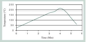
Peak reflow temperature should be <350°C in an air or nitrogen atmosphere (<500ppm 02), with a linear ramp up to 30°C above liquidus temperature. These profiles are recommended to the user as starting points, and should be optimized by the user to meet their individual process needs.
