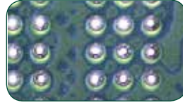
Ball Mount After ball mount, flux and ball position are good
