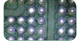
Post DI W Clean No missing ball and no flux residue
