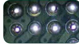
Post Reflow No missing ball and flux residue is clear
