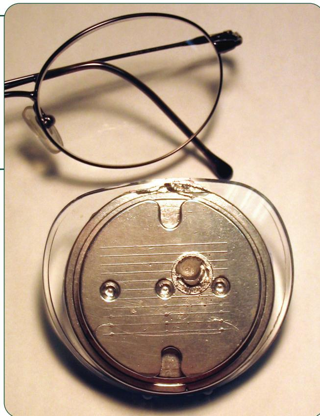
The surfacing block is then mounted in a chuck and is used to protect the lens during the grinding operation. After the grinding operation, plastic lenses are removed from the surfacing block by the inertia of knocking the surfacing block on a solid surface. Glass lenses are removed by dipping them into a hot water bath. When the alloy melts and the lens is separated from the surfacing block, the alloy settles to the bottom and is recovered by draining through a valve.
